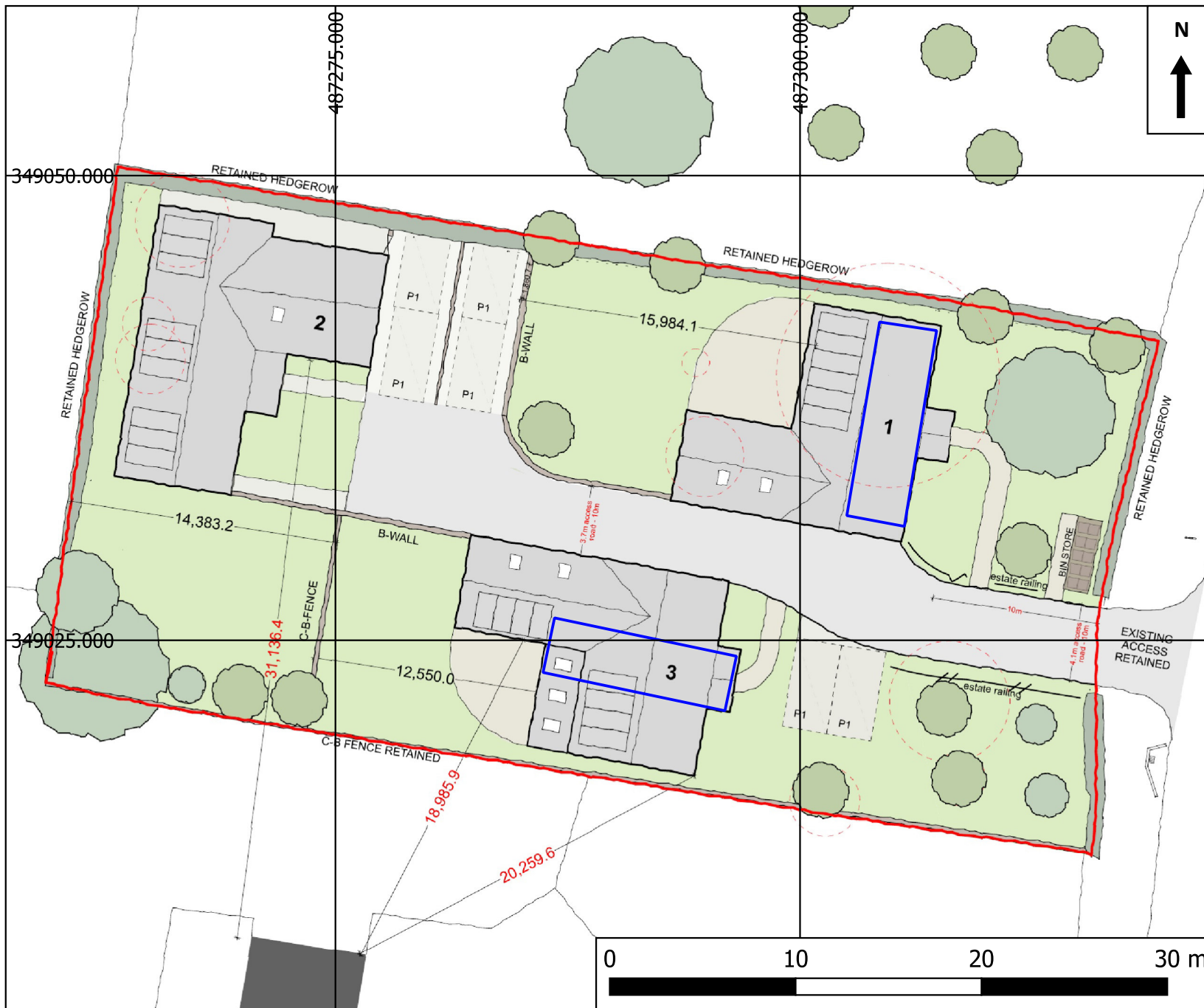
Figure 2: Plan of proposed development (outlined in red) and proposed trenches (outlined in blue). Base map provided by client
